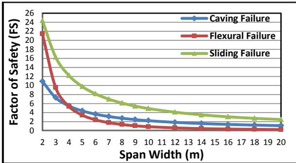
Figure 5.2. Curves relations safety factor and span width for 28 days age of pastefill
