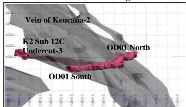
Figure 4.2. Model of Kencana-2 Vein Sub 12C Undercut 3 Ore Drive 01
