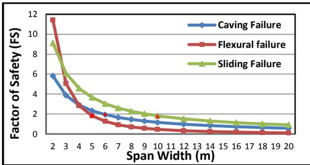
Figure 5.1. Curves relations safety factor and span width for 7 days age of pastefill
