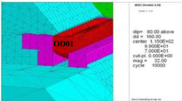
Figure 5.3. Failure type of pastefill block for 7 days curing time
