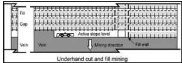
Figure 4.1. Scheme of underhand cut and fill mining method
