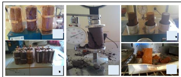
Fig.2 The stage of testing: a) the manufacture of the test object, b) curing process, c) testing of compressive strength (ucs test), d) weighing the specimen after testing, e) drying in an oven
